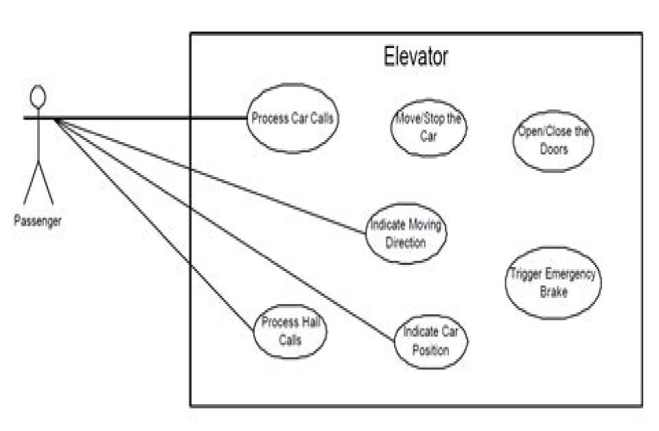
Use Case Diagram of Elevator System
