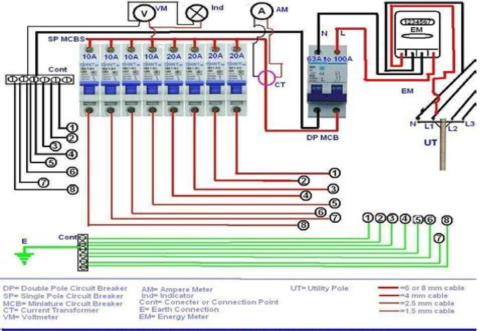
Distribution Board Wiring For Electrical Wiring / Home Wiring
