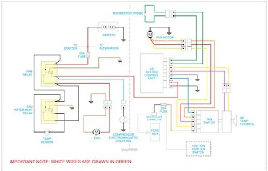
ALFA ROMEO SPIDER AC WIRING DIAGRAM
