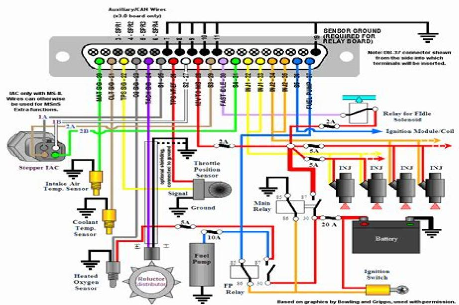
Note: Pin 24 can also be connected to the output of a half sensor, if the board is jumpered appropriately during assembly.
