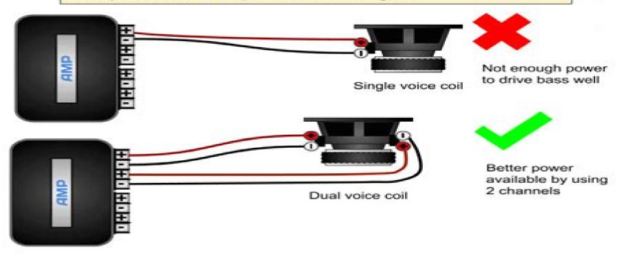
Maximum amp power: A DVC subwoofer can be used to get the maximum power from a 1 ohm stable amp by wiring two 2 ohm voice coils as a 1 ohm load.
