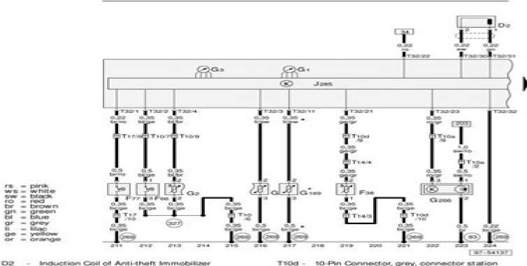
F38 - Ambient Temperature Switch F66 - Engine Coolant Level (ECL) Warning Switch F77 - Windshield Washer Fluid Level Warning Switch Sender for fuel gauge G1 - Fuel Gauge G2 - Engine Coolant Temperature (ECT) Sensor G3 - Engine Coolant Temperature (ECT) Gauge G169 - Fuel Level Sensor 2 G266 - Oil Level Thermal Sensor
