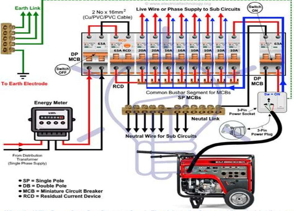
When the Utility Power Goes Out, Generator Supply Electricity to the Connected Electrical Appliances
