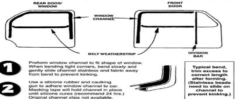
Original belt weatherstrip is stapled in place. Remove staples. Form and cut to length beltweather strips, leaving a little extra stainless to flatten. Install flattened stainless between channel and door to help hold it in place in corners.
