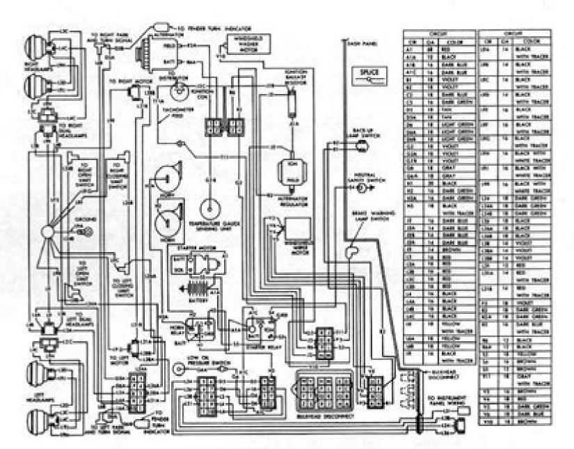
Engine compartment wiring diagram-Hemi-1967.
