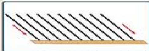
STEP #4 - Make sure connectors are properly lined up. Apply a small amount of silicone caulk to diameter of baluster where it meets baluster connector or insertion hole to insure a tight, movement free installation. Install balusters on bottom rail.
