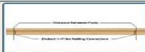
STEP #2 - Using step - 1 measurement, deduct 1/2" from total measurement for railing connectors. (If not using railing connectors, cut to step - 1 measurement). Cut both top and bottom rails.
