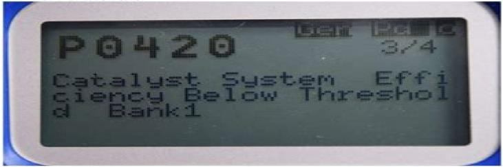
A P0420 code indicates a problem with the catalytic converter. The purpose of the catalytic converter is to break down harmful pollutants created during the combustion cycle. By using fine platinum and gold meshes to filter exhaust fumes, the catalytic converter is able to reduce the emissions expelled from the exhaust pipe.
