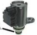
N/V = normally venting N/C = normally closed All Nissan valve bodies use the high resistance low coast solenoid. The Bosch, Nachi, and Mitsubishi high resistance solenoids can be freely interchanged. Always check the resistance on Infinity valve bodies to determine the correct low coast solenoid.
