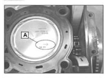
Push connecting rod / piston assembly out through top of cylinder bore of upper crankcase.
