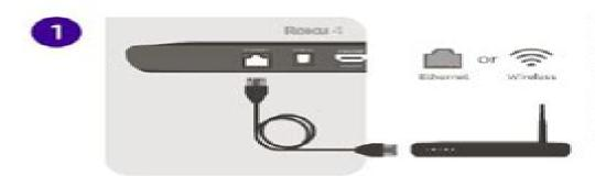
First, if you're going to connect to the internet via a wired connection, connect an Ethernet cable to the Ethernet port on the back of the Roku 4.
