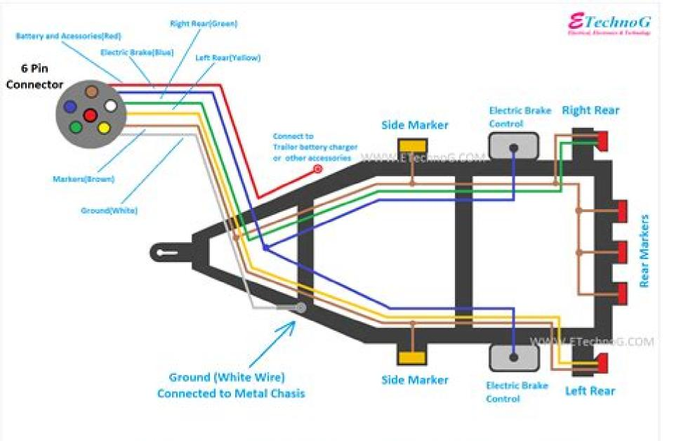
6 Pin/Wire/Way Trailer Wiring Diagram (with Light, Brake, Battery)
