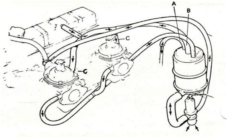
Fuel vapors from the TR6 gas tank are absorbed into this carbon canister filter when the engine is stopped. They are purged into the crankcase emission system and through the carburetors when the engine is running.
