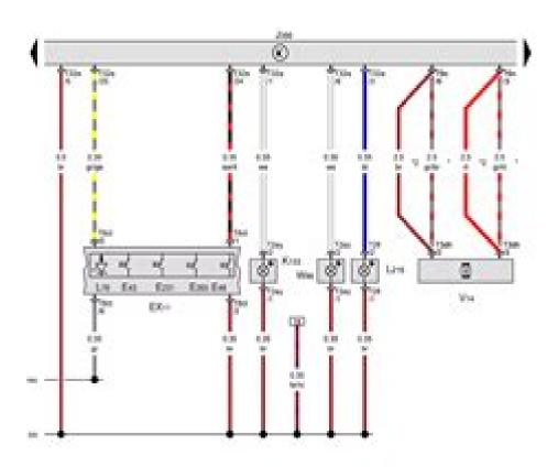
Exterior mirror adjuster, Driver door control unit, Central locking SAFELOCK function warning lamp, Light for driver side interior door handle illumination, Left window regulator motor, Light for driver door background lighting
