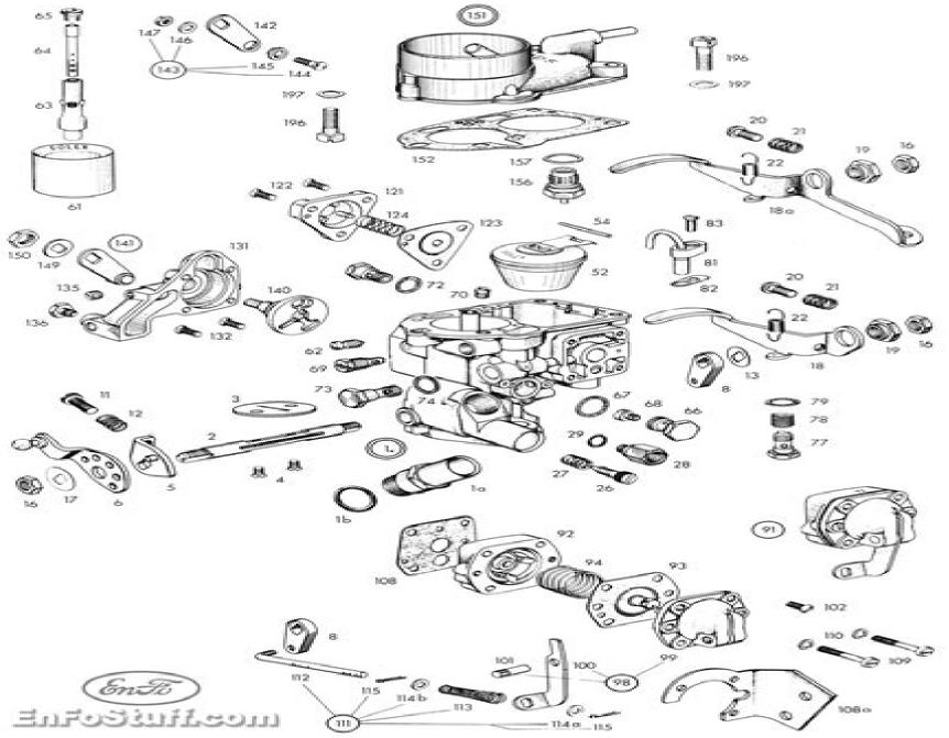
Exploded view of the Solex 32 PICBA carburetor used on the Taunus 17M.
