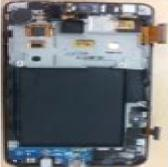
Separate all connector ribbons from the PBA. Separate the PBA from the Front.
