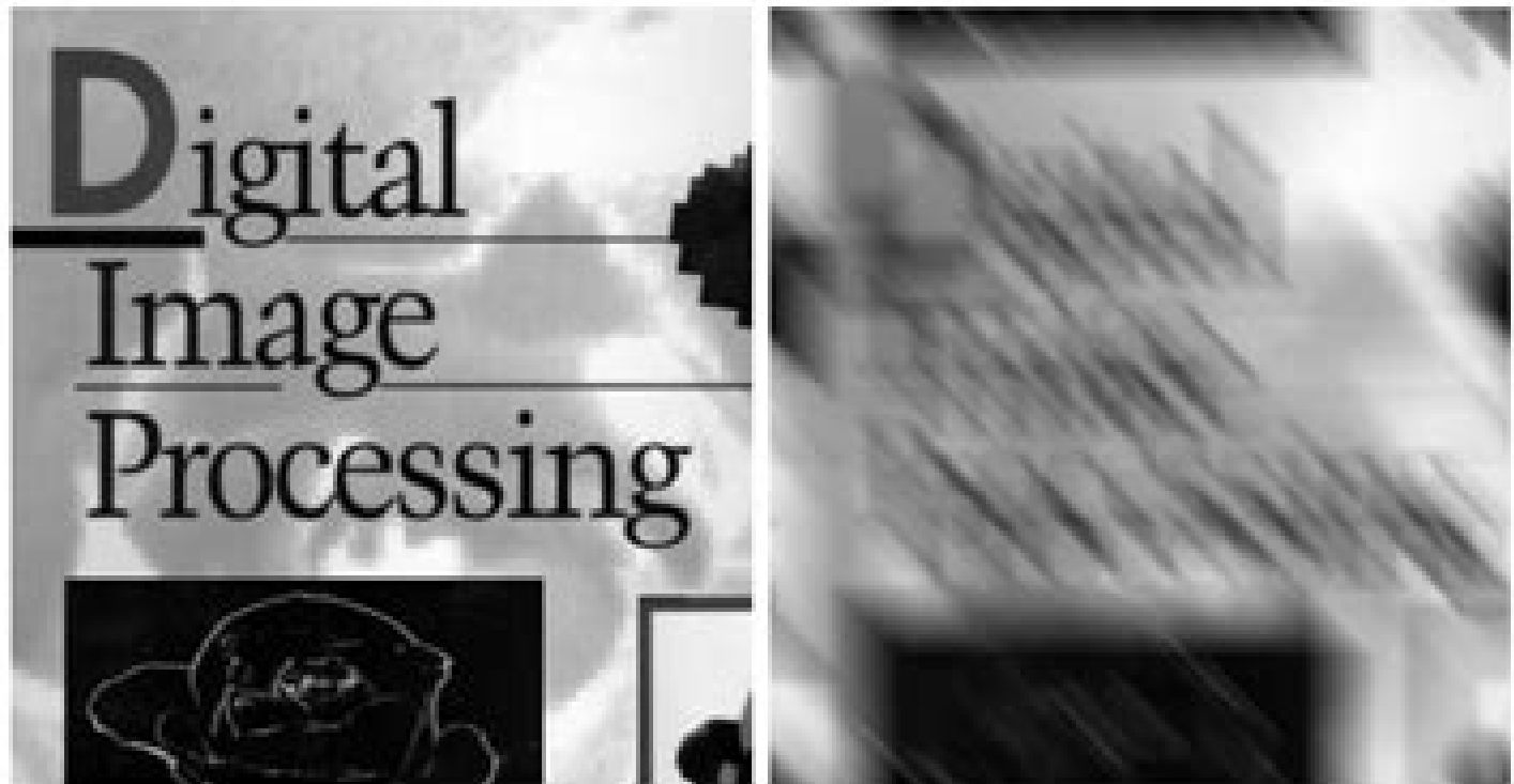
FIGURE 5.26 (a) Original image. (b) Result of blurring using the function in Eq. (5.6-11) with a = b = 0.1 and T = 1 .
