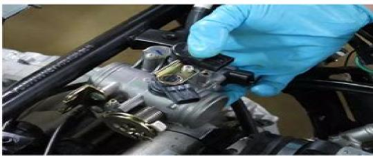
Remove the throttle out of the air box and intake boots.
