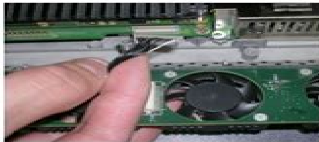
Figure 8-68 Disconnecting the Fan Cable from the BEP
