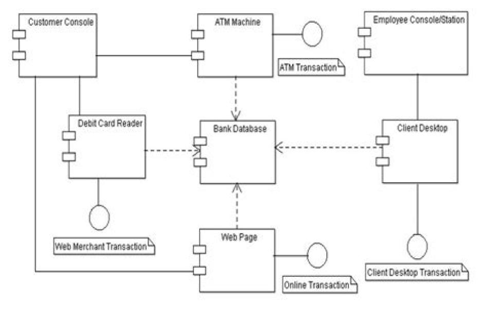
dig.Component diagram of ATM System
