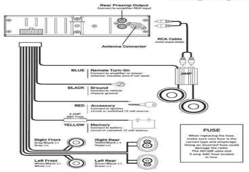
Caution – Do not attach any speaker leads to ground as severe damage will occur.
