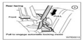
Pull on the shoulder belt until all of the belt is fully extended. At this time, the seat belt retractor is in the automatic locking mode (child restraint mode), it reverts back to emergency locking mode when the seat belt is fully retracted.
