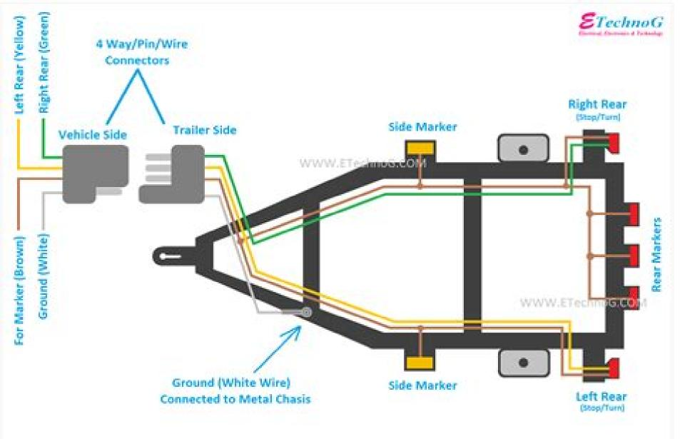
4 Pin/Wire/Way Trailer Wiring Diagram (with Light)
