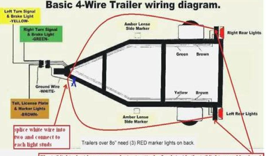
The tail lights dont have a ground wire to attach - Look inside the tail light assembly of each tail light and you will see that the lights are ground via contact with the mounting studs!
