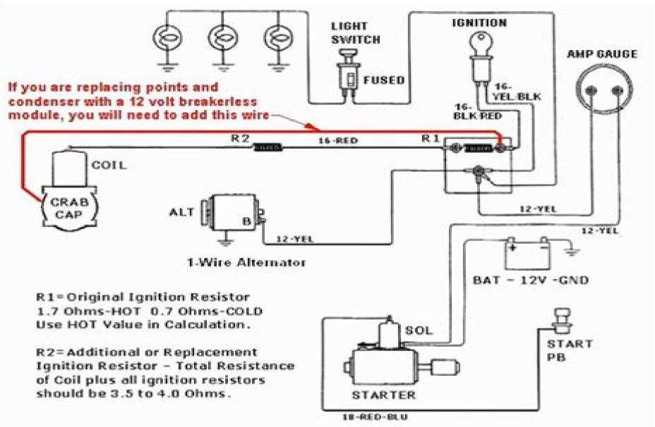
1-Wire Alternator 12-VOLT CONVERSION - FORD 8N FRONT DISTRIBUTOR 1947 TO 1950
