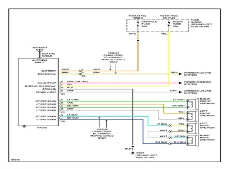
Fig. 7: Mono Radio Circuit
