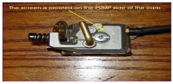
The primary screen is located on the PUMP SIDE of the carburetor. Remove the single screw located in the middle of the pump cover and carefully lift off the cover & rubber gasket, noting the position of the gasket. When re-assembling the carb make sure the pump diaphragm or gasket is situated correctly, then re-install the pump cover and screw.
