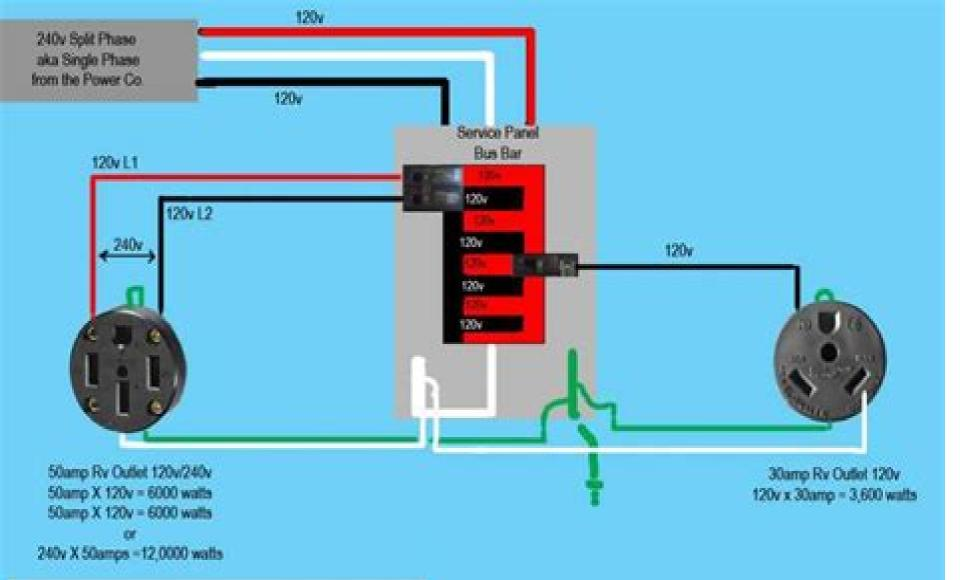
Each Line fed by the 50amp Breaker is capable of 50amps BUT since they are tied together by the Breaker- if one Line sees more than 50amps the Breaker trips both lines
