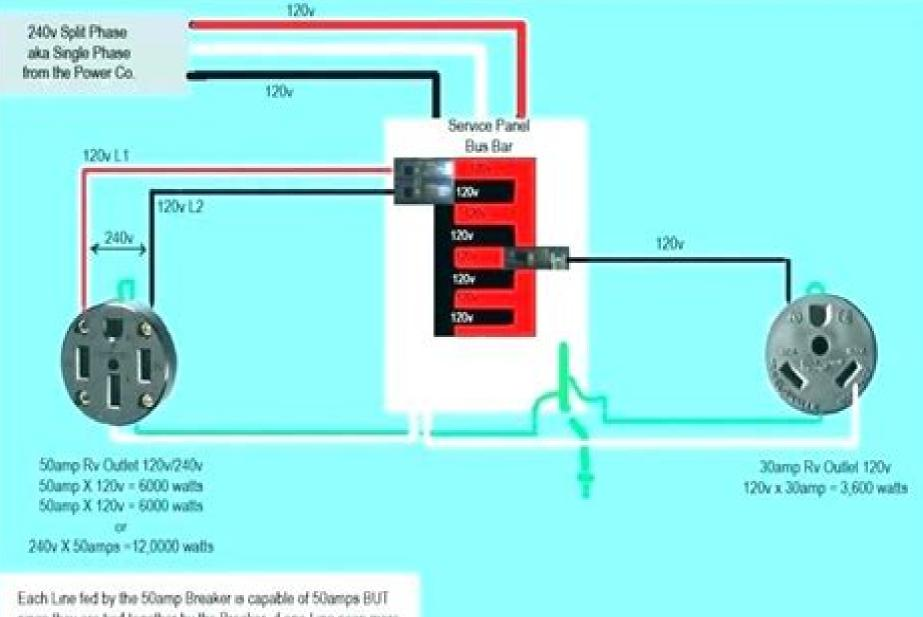
Each Line fed by the 50amp Breaker is capable of 50amps BUT since they are tied together by the Breaker- if one Line sees more than 50amps the Breaker trips both lines.
