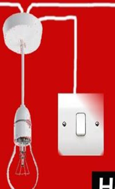
wiring 1 way switch ceiling rose
