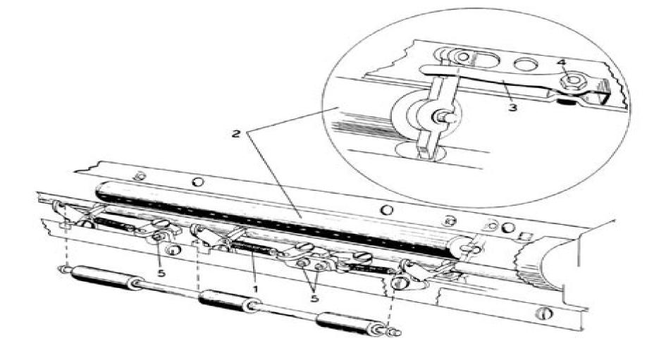
Proper paper feed depends almost entirely upon the condition of the platen and the feed rolls. If these are in good condition, your paper feed problems are about solved. <u>Review</u> the platen and feed roll pages of the General Information Section. This information will help you determine if a new platen or new feed rolls are necessary.
