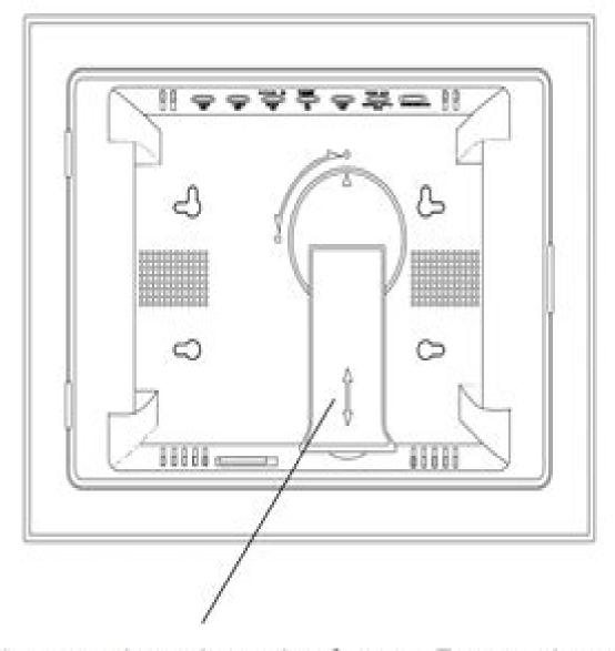
Pull out the stand to place the frame. Rotate the stand to position the frame vertically or horizontally. Adjust the stand's length to obtain the desired vertical or horizontal viewing angle.
