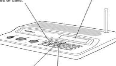
Tune — lets you tune for new and unlisted frequencies starting from a specified frequency.
