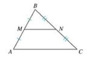
If a line bisects one side of a triangle and is parallel to a second side, then it bisects the third side and therefore is a midsegment.
