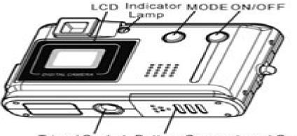
Tripod Socket Battery Compartment Cover
