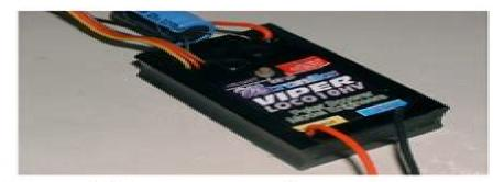
The VIPER ESC's do not have directional constant brightness lightness output controls. Use the RCS # REV-LT to have automatic constant brightness directional lighting. SETTING UP VIPER FOR THE 1st TIME
