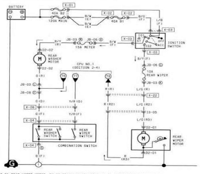
D2-01 REAR WIPER MOTOR D2-02 REAR WASHER MOTOR 13-05 CONNECTOR BETWEEN REAR NO.2 (R2) AND REAR NO.3 (R3)
