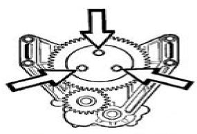
Remove the idler gear from the oil pump housing.
