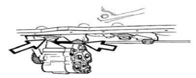
Remove the bolts for the front main bearing cap and lift down the lubricating oil pump together with the main bearing cap.
