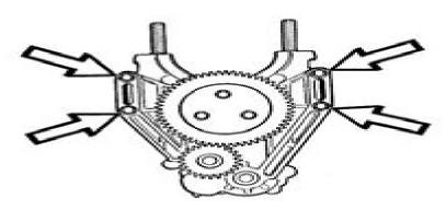
Remove the lubricating oil pump from the main bearing cap.
