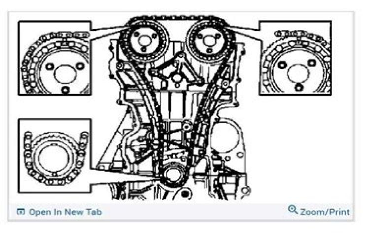
Make sure the three timing marks on the timing chain are exactly aligned with the marks on the exhaust camshaft sprocket, intake camshaft sprocket, and crankshaft sprocket respectively.
