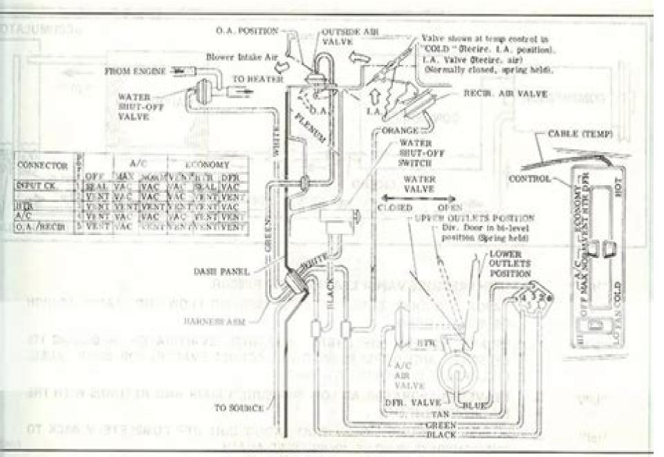
Fig. 18-4-C60 A/C Vacuum Diagram
