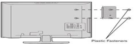
2 Insert the 2 Plastic Fasteners (supplied) into the holes. then press in the head of the fasteners using your finger until they click.
