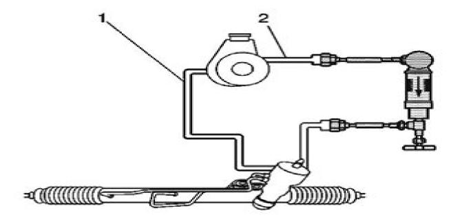
Fig. 3: Testing Rack and Pinion System Pressures Courtesy of GENERAL MOTORS CORP.
