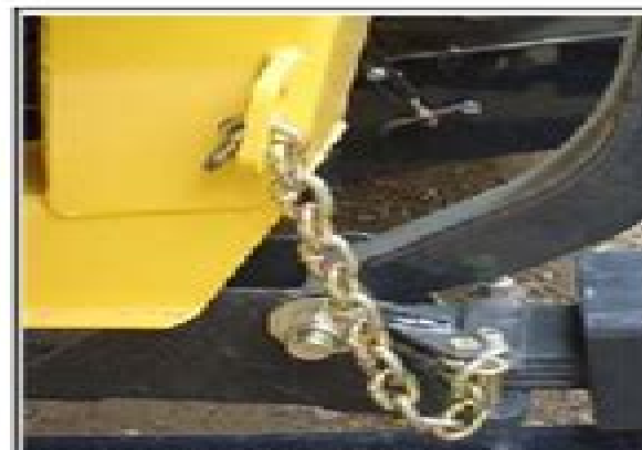
Loose Restrainer Chain
