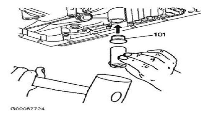
Fig. 4: Installing Oil Filter Seal Courtesy of GENERAL MOTORS CORP.
