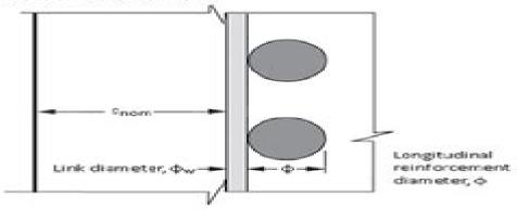
You are required to set a minimum value for the nominal cover,  $c_{nom, w}$  for each column in the column properties.
