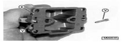
Install the two slow speed jets (V) into the float chamber (E) and tighten to 0.7 N-m (6 lb-in.).
