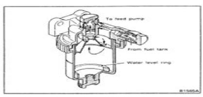
The sedimenter type water separator separates gas oil and water centrifugally by taking advantage of their difference in specific gravity.
